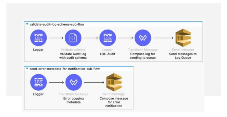
An ingest pipeline from SQS to log analytic platform can be built whether in MuleSoft itself, any serverless app or any other platform. For error notification, the necessary attributes can be sent a queue, on further reading of the message, a decision can be taken whether to send a notification or retry the message.
